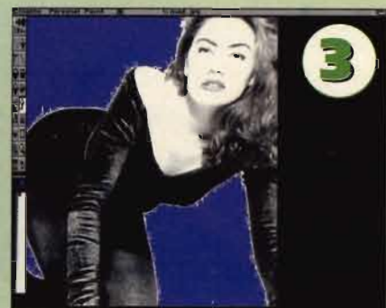
3 Flood fill the background with some solid colour. This isn't essential but it will make things easier later on if you do, especially if you want to strip in a new colourful background.
